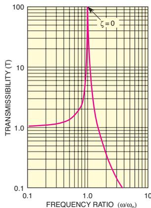
Figure 2. Transmissibility of a Simple Harmonic Oscillator.
