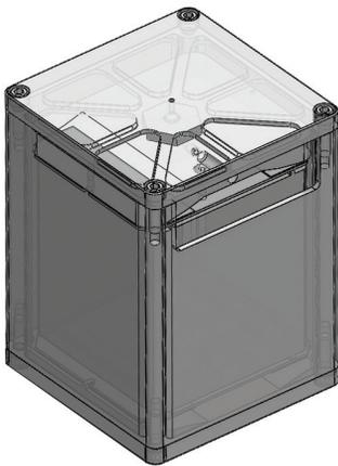
**Figure 2:** Schematic of Newport vibration absorber used in tuned damping table systems US patents 8,857,585 et al.modes of table vibration.
