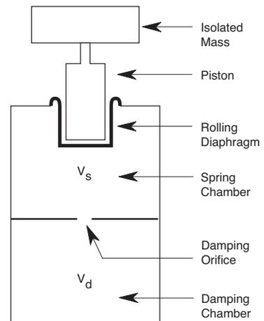
Figure 19: A conventional pneumatic isolator with damping.
