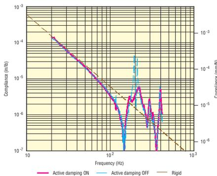
Dynamic compliances near the corner of the table. Red line: damping on; Blue line: damping off, dots: rigid body line. Table size: 8ft x 4ft x 12in.
