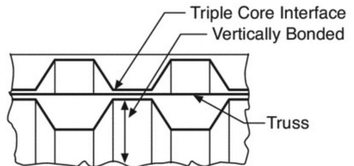
Figure 5: Trussed core design offers superior rigidity
