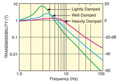
**Figure 17:** Transmissibility plot shows damping effects.
