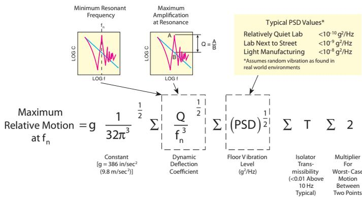
Figure 1. Formula for determining the maximum relative motion between two points on an isolated table top from any compliance curve. Table tops supported by rigid stands (or legs) would have a larger relative motion value.
