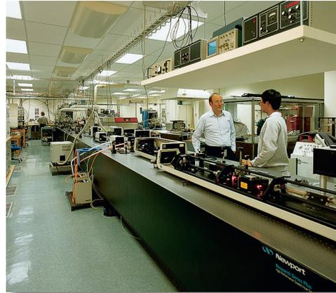
Figure 1: Newport table systems minimize the relative motion of a large array of sensitive scientific and production equipment
