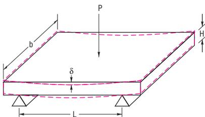
Figure 2. Static deflection for a point load P applied at the center of a panel supported at the recommended isolator locations.
