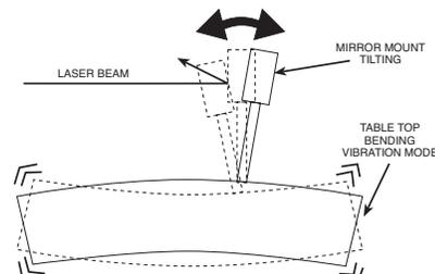
Figure 2: Table top bending is the most significant cause of beam deflection.
