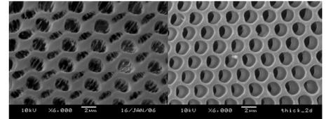
The Nanostructures shown in the images above were built on and imaged with a SmartTable. The image on the left was built with SmartTable damping disabled. The image on the right was built with SmartTable damping enabled. Source for images: Steven E. Kooi, Ph.D. Research Engineer, Institute for Solder Nanotechnologies, MIT
