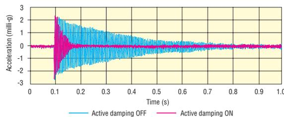
Compared with passive damping technologies, IQ damping provides much more accurate and timely compensation across the entire working ranges of the actuator sensor pairs, delivering a quiet tabletop surface for any challenging applications.
