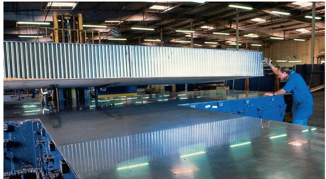
Figure 6: These precision platens allow the manufacture of large tables on a single, ultra-flat surface instead of multiple granite platens, which can compromise end-to-end flatness.
