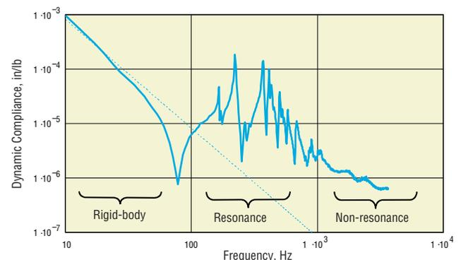
**Figure 1:** Typical corner compliance of an optical table without any special means of damping
