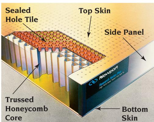
Figure 2: Honeycomb core construction creates exceptionally rigid platform for precision optical experiments
