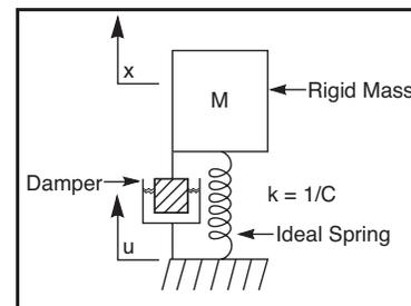
Figure 3. Damped Simple Harmonic Oscillator
