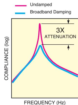
Featuring 6 precision tunable dampers, RS4000 brings the best passive damping performance to your applications that require critical level of damping. The 6 dampers are designed specifically to target majority of the resonances of the table. The result is an ultra quiet tabletop that's ideal for critical applications such as live cell imaging, high resolution imaging, interferometry, experiments with long exposure time and so on.
