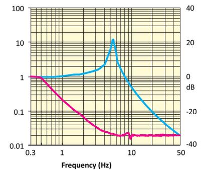
— Passive (with VIBe-X Isolators Only) — Active (With Guardian active modules and VIBe-X isolators)
