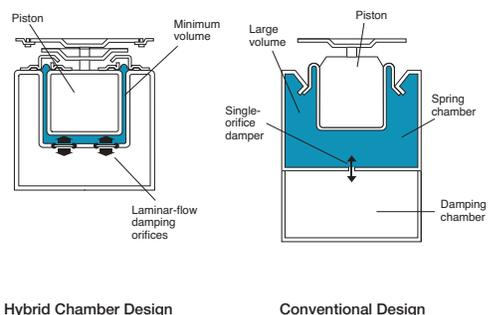
Figure 20: Damping chamber
