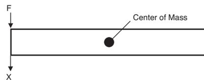
Figure 3. In practice, table top compliance is tested by striking the table edge, and measuring table top response in the same location.
