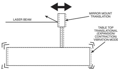
Figure 1: Translational motion of the table top does not affect even sensitive systems.
