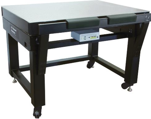
The Guardian workstation includes two active isolation modules each contains 3 sensors and 3 actuators to actively sense and compensate for vibration in six degree of freedom real-time. It not only removes the resonance response inherent to the passive system, but provides up to 34 dB (50 times) additional isolation. Isolation starts at 0.5 Hz and reaches 20 dB (10 times) at 1.5 Hz. It vastly outperforms not only the passive spring-based systems, but also the best pneumatic workstations.
