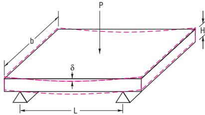
Sandwich structures for vibration isolation tables are stiffer than solid tables of equal weight. For the same weight, the fundamental frequency of a sandwich table is higher than that of a solid table. Although the bending behavior of a sandwich table is complex, the following simple approximations are useful.
