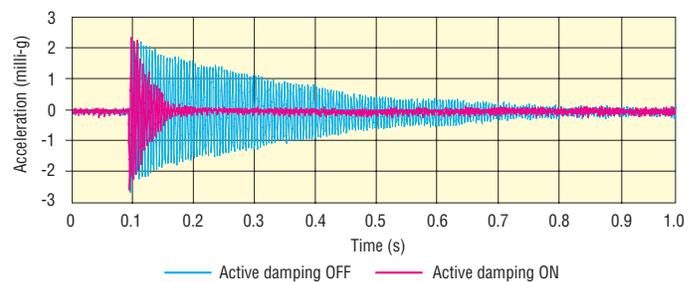
**Figure 8:** Transient attenuation near the corner of the table. Red line: damping on; Blue line: damping off. Table size: 8 ft x 4 ft x 12 in.
