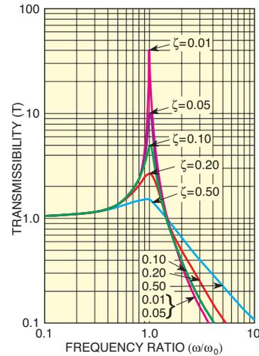
Figure 4. Transmissibility of a damped oscillator system with various values of the damping coefficient ( $\zeta$ ).
