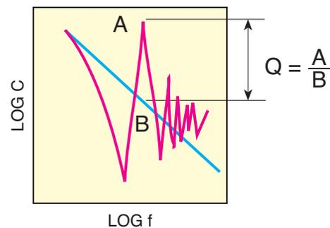
Figure 6. Maximum amplification at resonance (Q).
