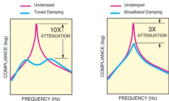
**Figure 1:** Newport tuned dampers (left) concentrate damping where it's needed most, at the frequencies of dominant resonance modes. Since broad-band dampers (right) are designed to provide moderate damping over a wide range of frequencies, they are not as effective at damping the dominant modes of table vibration.
