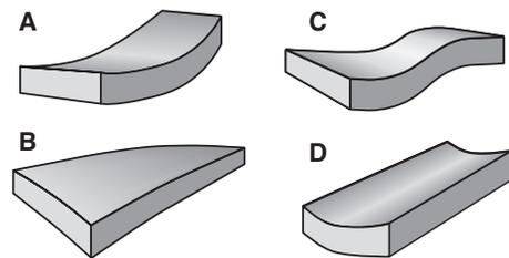
Figure 3. Vibrational modes of table top associated with compliance curve in Figure 2.
