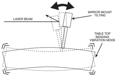
Newport's Maximum Relative Motion formula provides an excellent approximation of maximum (worst-case) table top deflection. This technical note explains and quantifies the relationship between Maximum Relative Motion and actual beam deflection in real-world applications.
