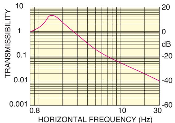
For example, given a system with a 2 Hz natural frequency; and thus a transmissibility of one at 2.8 Hz (1.41 x 2); the transmissibility at 28 Hz would be -40 dB, or 0.01. Horizontal isolation in a Newport isolator is achieved by use of a pendulum system. The behavior of the pendulum horizontal isolator is basically the same as that of the vertical pneumatic isolator. In this case, the pendulum natural frequency is given by:
